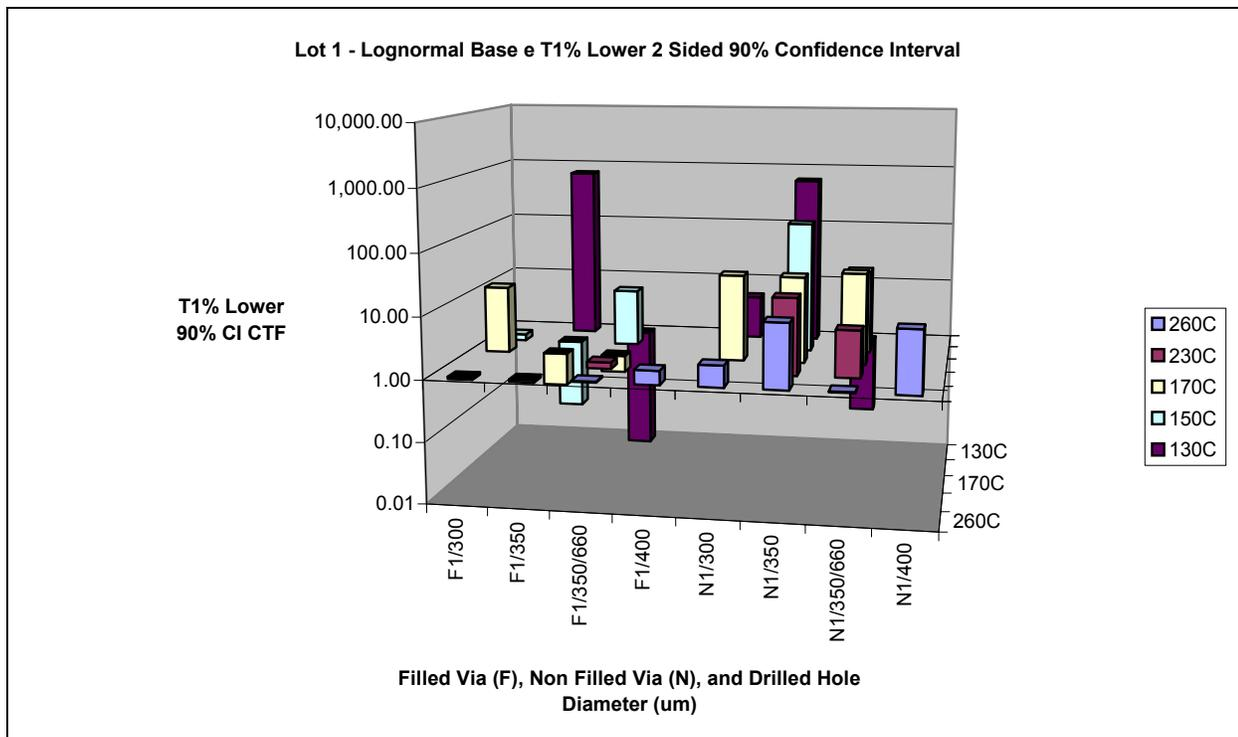
**Graph 1** – Lot 1, filled vias are on the left side, non-filled vias are on the left side. Within each via type data runs from smallest hole on the left to largest on the right.
