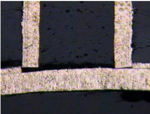
**Photo 2** – Microsection of a filled via from Lot 1 enlarged to show the plating in and over the filled via in pad configuration.
