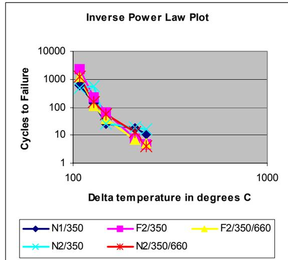
**Graph 3** – Log-Log plot consistent with an inverse power law relationship. Note the upturn, i.e., lower slope above Tg. See Graphs 7-9 for more detailed plots of this data.
