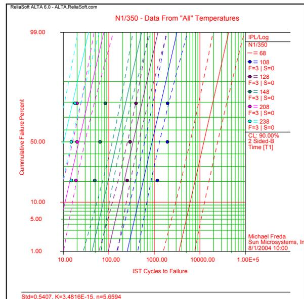
**Graph 4** – Log-Log plot of life versus stress analysis using the inverse power law. All five testing temperatures used for this Graph.
