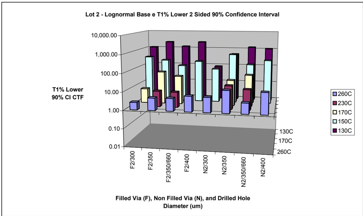
**Graph 2** – Lot 2, filled vias are on the left side, non-filled vias are on the left side. Within each via type data runs from smallest hole on the left to largest on the right.
