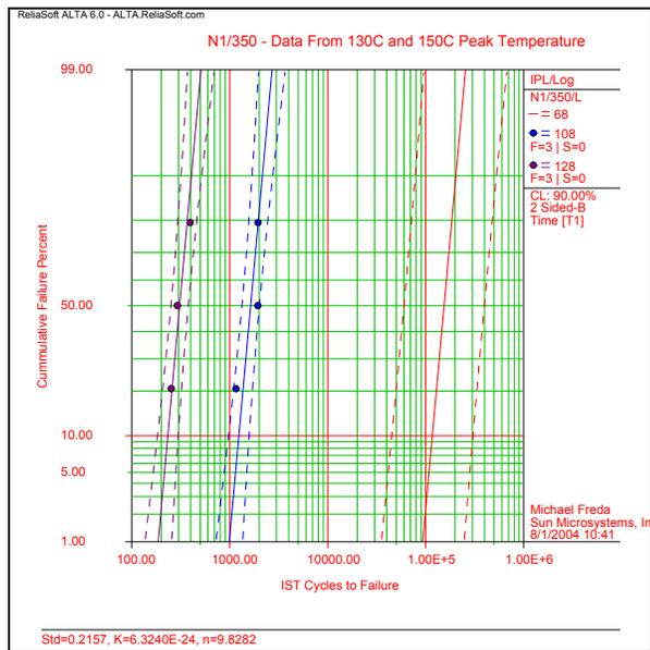
**Graph 5** – Log-Log plot of life versus stress analysis using the inverse power law and only CTF data from testing at 130°C and 150°C, i.e., well below Tg.
