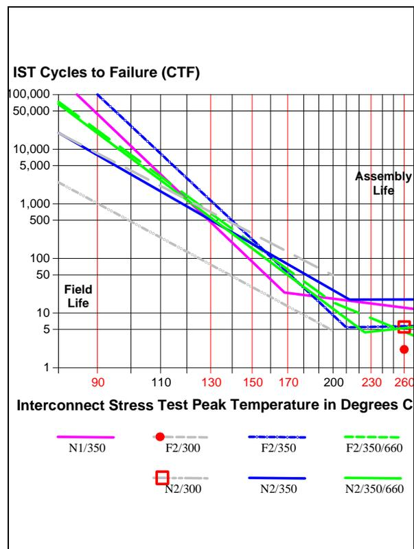
**Graph 7** – IPL plot temperature stress versus CTF. N1/350, F2/300, F2/350, F2/350/660, N2/300, N2/350, and N2/350/660 data plotted.
