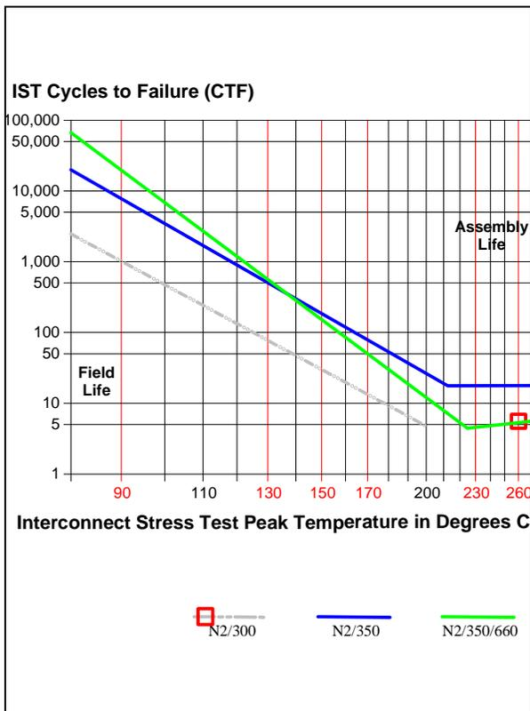
**Graph 8** – IPL plot temperature stress versus CTF. Only Lot 2, non-filled via data, i.e., N2/300, N2/350, and N2/350/660 data plotted.
