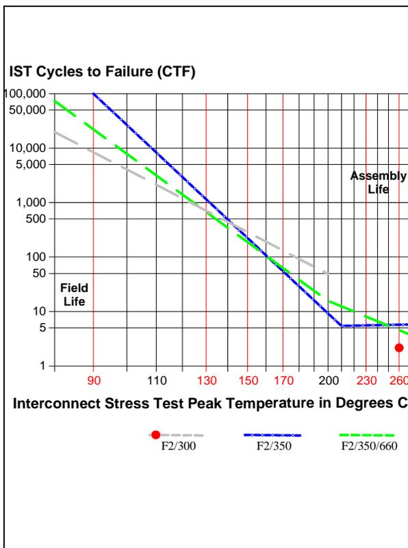
**Graph 9** – IPL plot temperature stress versus CTF. Only Lot 2, filled via data, i.e., F2/300, F2/350, and F2/350/660 data plotted.
