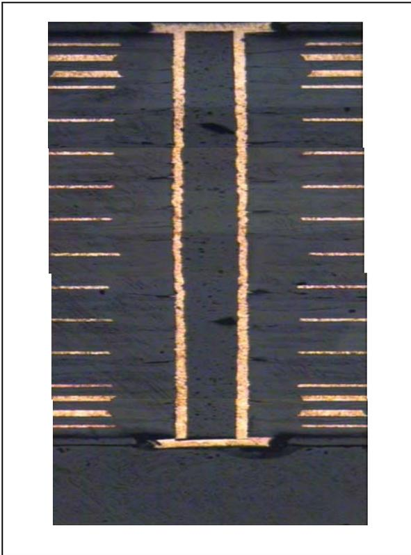
**Photo 1** – Microsection of a filled via from Lot 1. Note the plating over the filled via at the top and bottom of the microsection to form the via in pad structure. Failure occurred during 2x preconditioning at 260°C.
