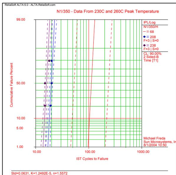
**Graph 6** – Log-Log plot of life versus stress analysis using the inverse power law and only CTF data from testing at 230°C and 260°C, i.e., well above Tg.
