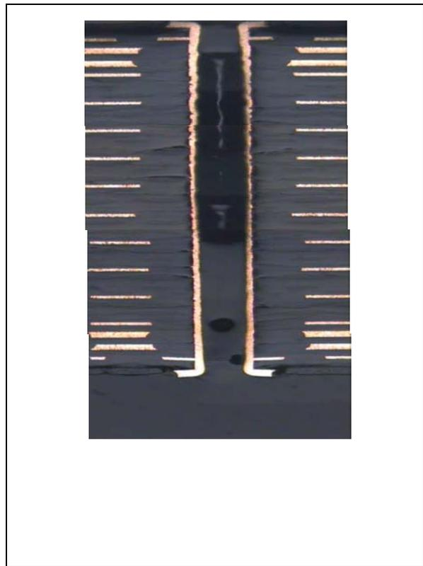
**Photo 4** – Microsection of a non-filled via from Lot 1. Failure occurred after 2 preconditioning cycles at 260°C and followed by 792 CTF at 130°C.
