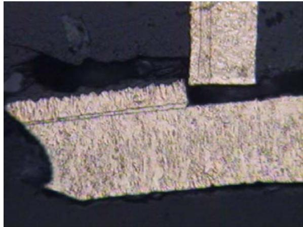
**Photo 3** – Microsection of a filled via from Lot 1. Note the lack of copper plating wrap around at the corner due to aggressive planarization. This may be the cause of the early life failure of this IST coupon.
